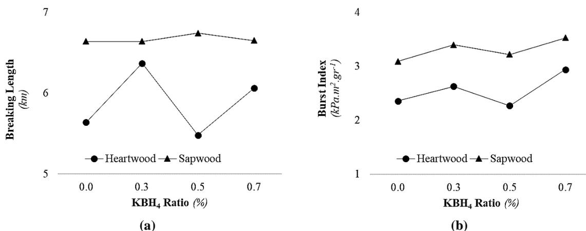
Figure 1. Effects of  $\text{KBH}_4$  on breaking length (a) and burst index (b) of *P. pinea* heartwood and sapwood pulps
