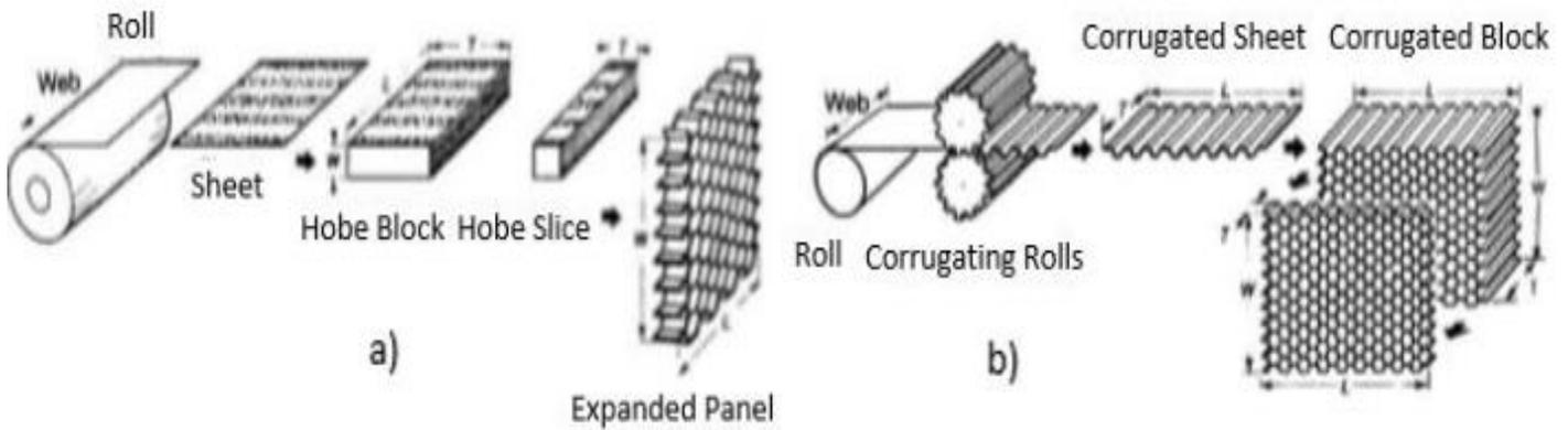
**Fig. 3.** Traditional honeycomb core manufacturing methods a) Expansion method of core manufacturing, b) corrugation method of core manufacturing [12].
