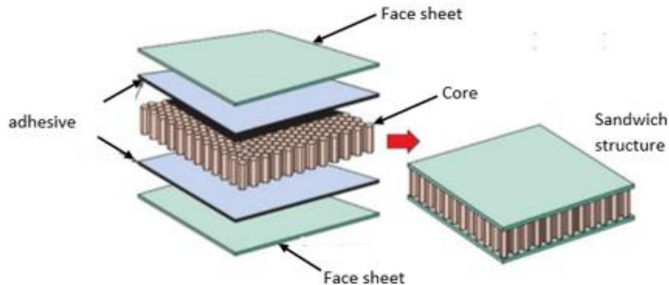
**Fig. 1.** Basic schematic view of sandwich structure [3]
