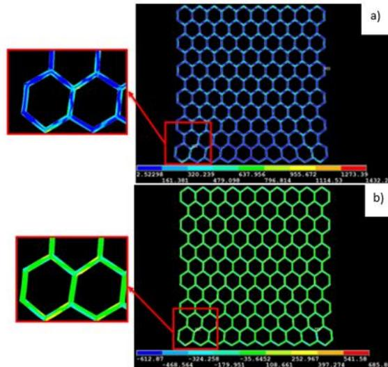
**Fig. 6.** a) Von-Mises stress distribution on model, b) Shear stress distribution on model
