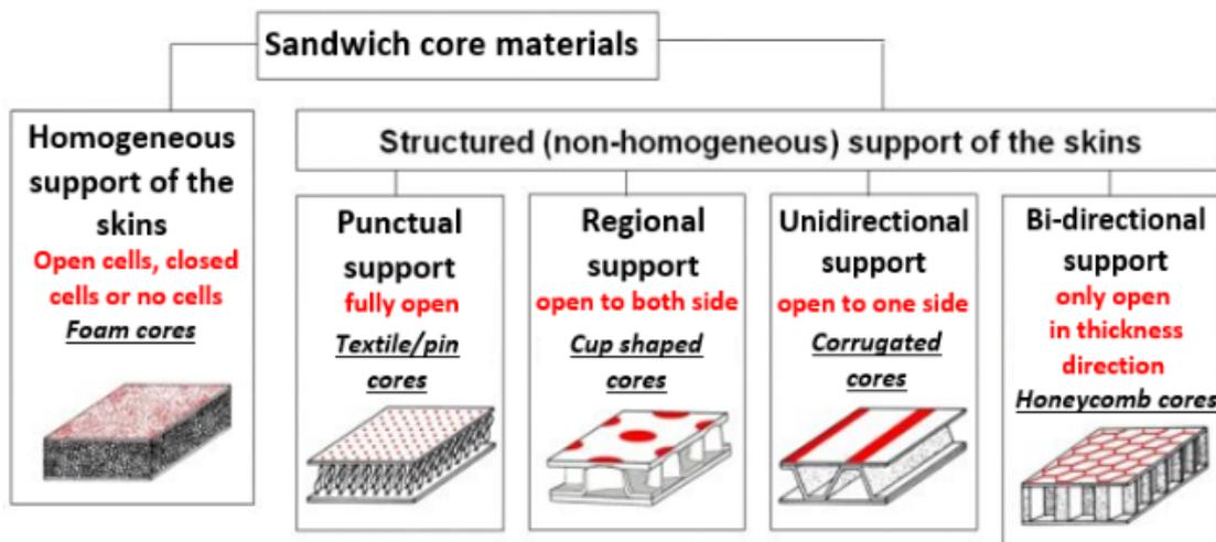
**Fig. 2.** Classification of sandwich core materials [6]
