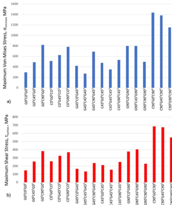
**Fig. 7.** Change of stresses depend on layer sequence, a) Maximum Von-Mises stress vs layer sequence, b) Maximum shear stress vs layer sequence
