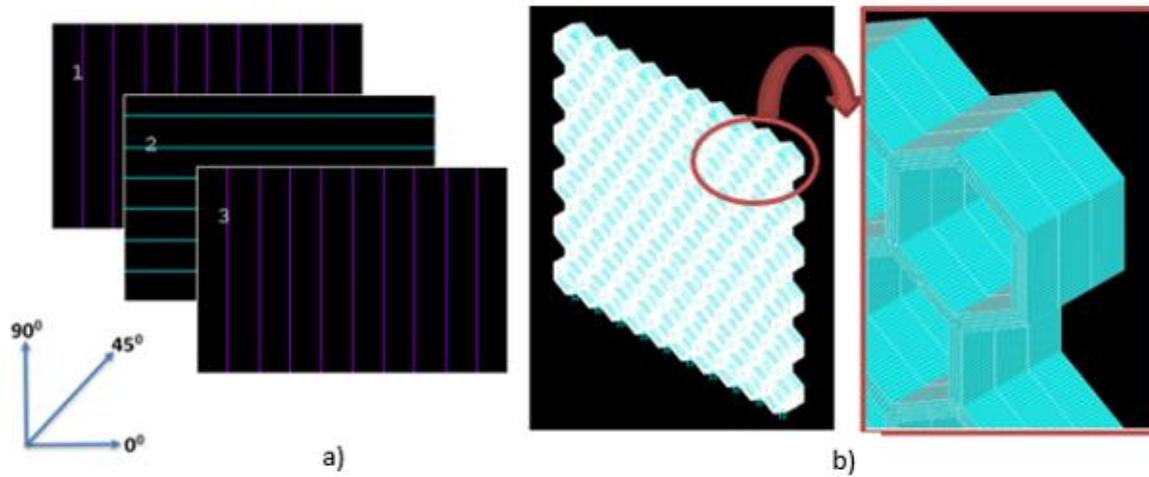
**Fig. 4.** a) Schematic view of a layer sequence of  $90^{\circ} - 0^{\circ} - 90^{\circ}$ , b) meshed model
