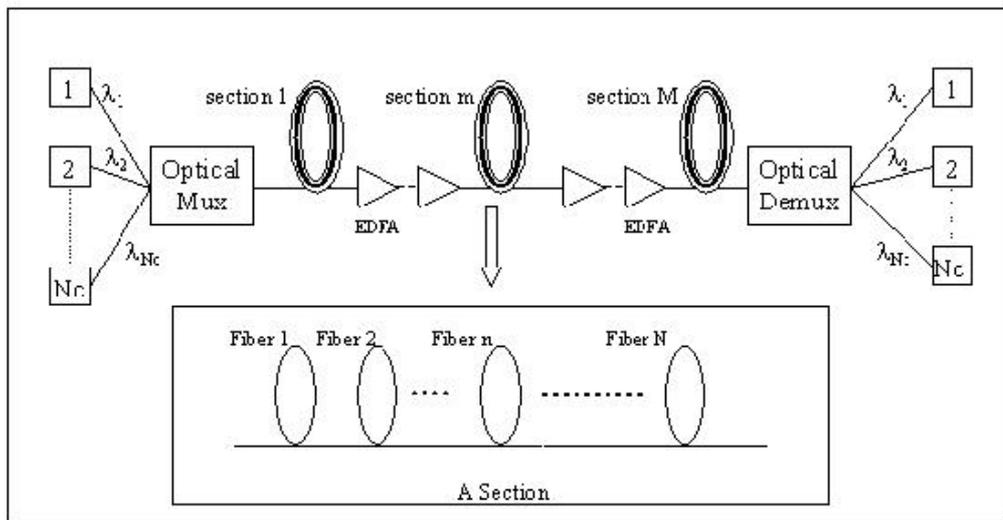
Fig. 1: Configuration of the optical transmission system
