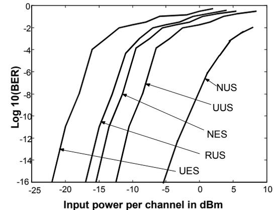
Fig. 6: Bit error rate characteristics for varying input power; UES: uniform dispersion and equal spacing, NES: nonuniform dispersion and equal spacing, UUS: uniform dispersion and unequal spacing, NUS: nonuniform dispersion and unequal spacing, RUS: repeated unequal spacing
