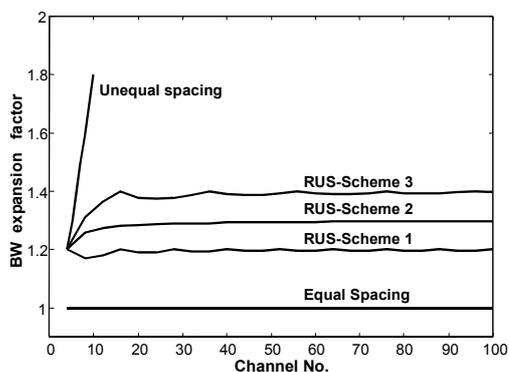
Fig. 2: Bandwidth expansion factor with increasing number of channels
