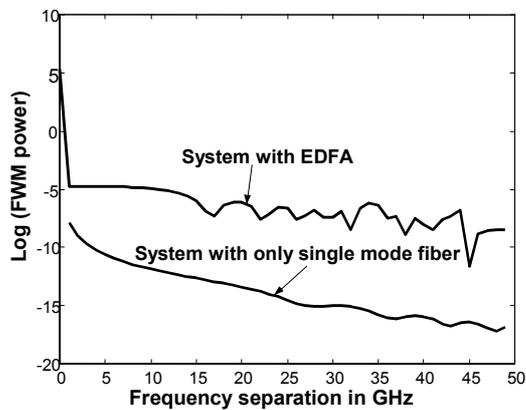
Fig. 4: Generation of FWM power in EDFA
