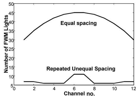
Fig. 3: Number of FWM lights produced in different channel positions for US and RUS schemes
