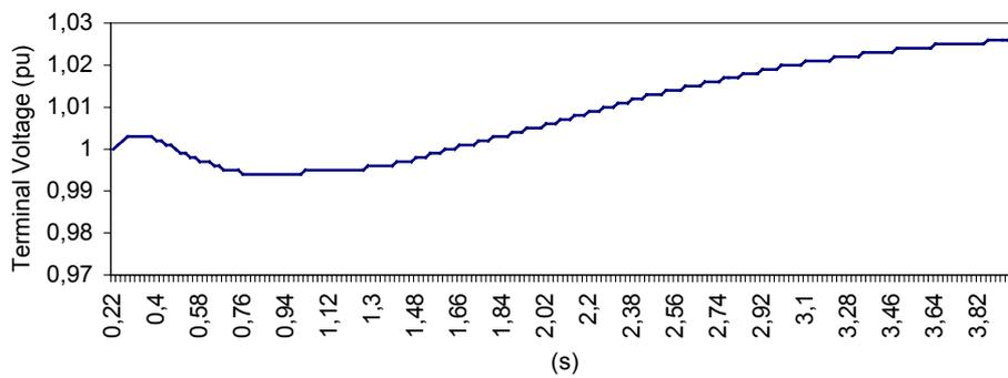
Figure 5. Transient Stability analysis for the constans  $K_A=42,03$  and  $T_A=0,198$
