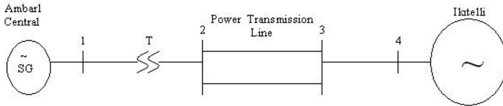
Figure1. One machine energy system chosen between Ambarlı Central and İkitelli
