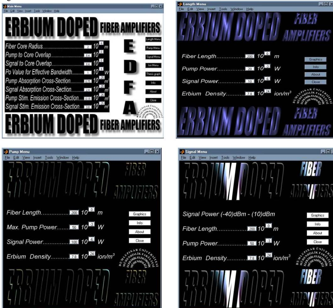
Figure 4. The main and sub menus of the simulation program.
