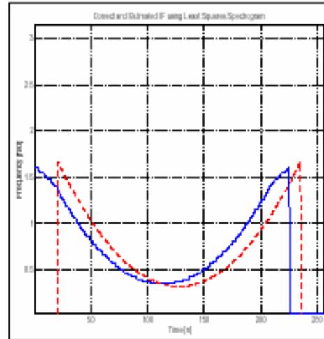
Fig. 3. Correct (dashed line) and estimated (solid line) IF by spectrogram combinations.
