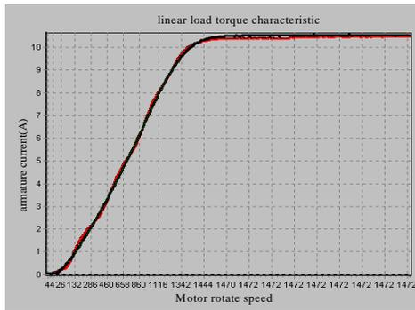
(b) Linear Load Torque Curve
