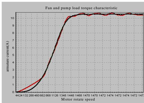
(c) Fan and Pump Load Torque Curve
