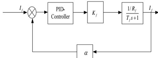
Figure 6 the Mathematic Model of Exciting Current Controller
