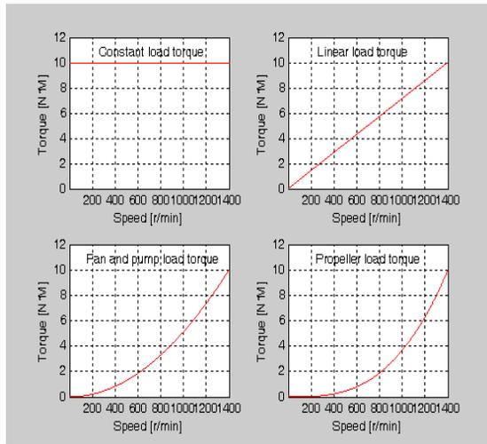
**Figure 3** Typical Load Torque/Speed Curves
