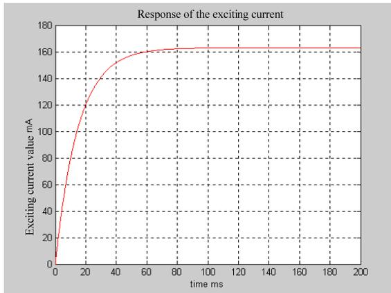
Figure 7 Response of the Exciting Current for PI-Controller
