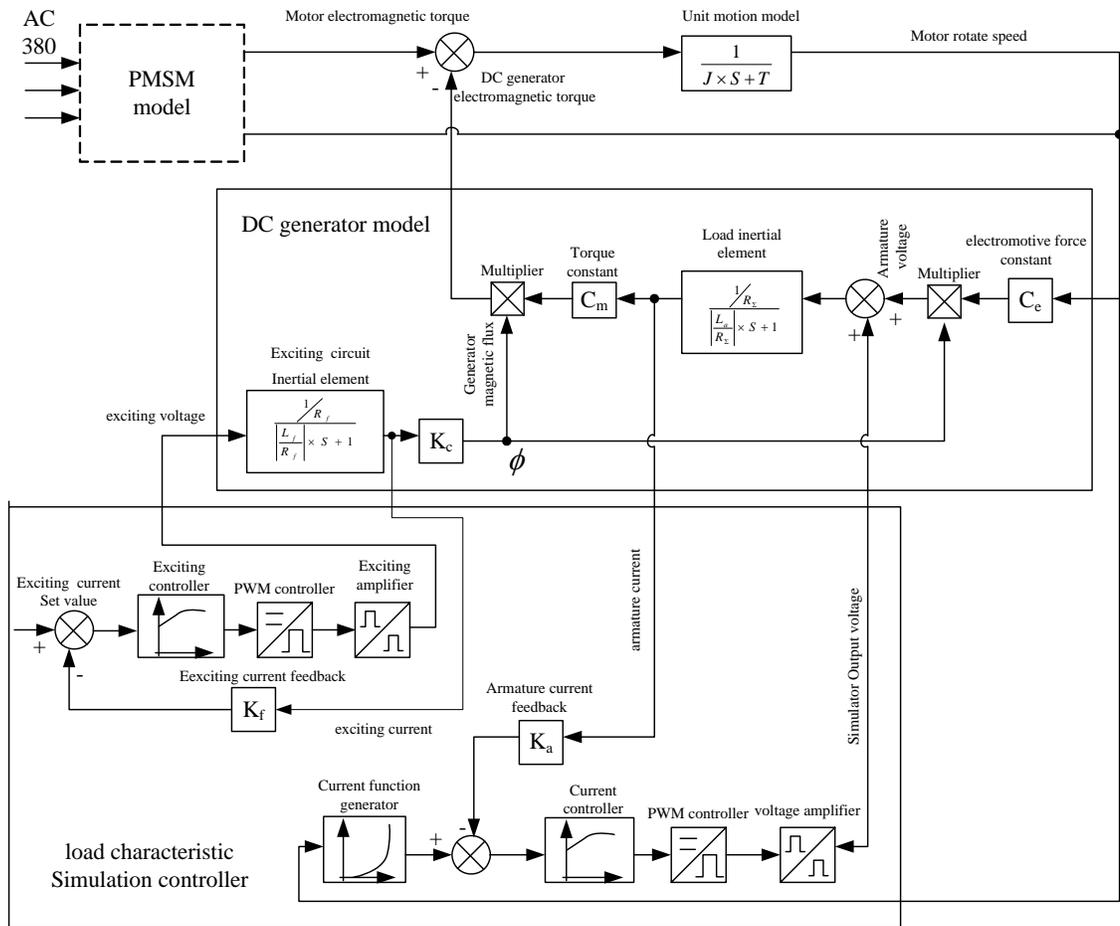
Figure 5 the Block Diagram of Load Torque Simulator
