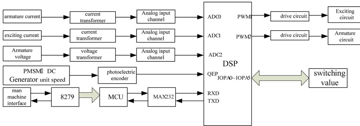
Figure9 the Integrated Architecture of Load Simulator Controller
