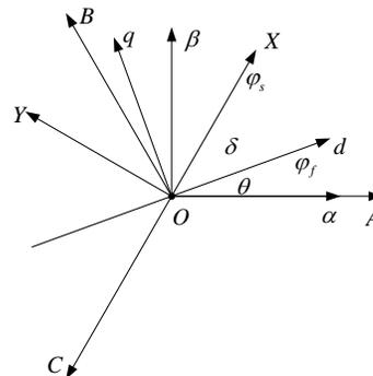
**Figure 1** the Reference Frames Used in DTC
