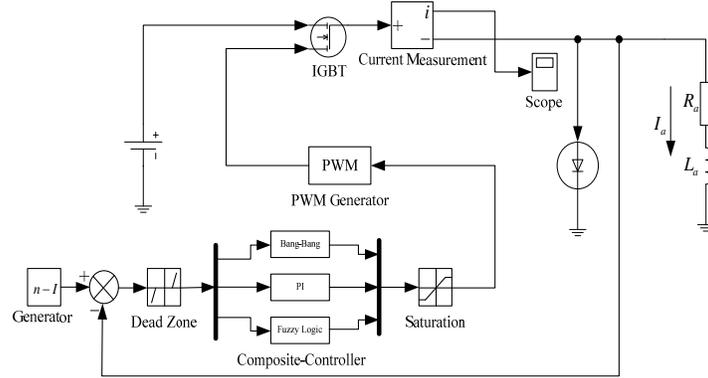
**Figure 8** the Block Diagram of Composite-Controller for Armature current
