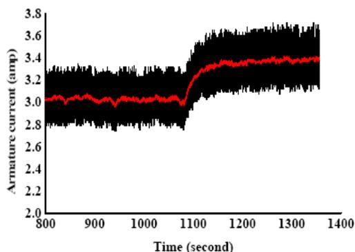
**Fig. 13:** Variation of armature current with step load
