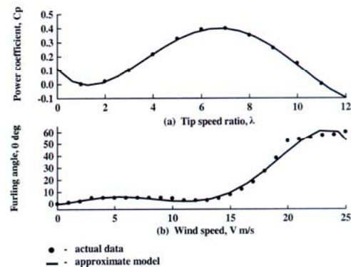
**Fig. 1:** (a) Power coefficient as a function of tip-speed ratio. (b) Furling angle versus wind speed.
