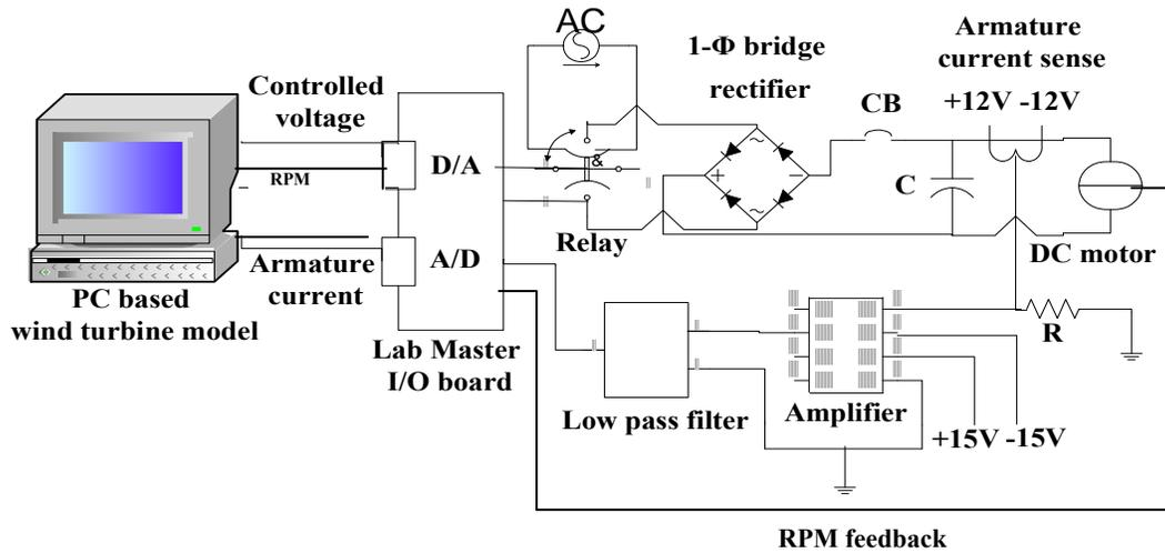
Fig. 5: Schematic of the wind turbine section of the emulator
