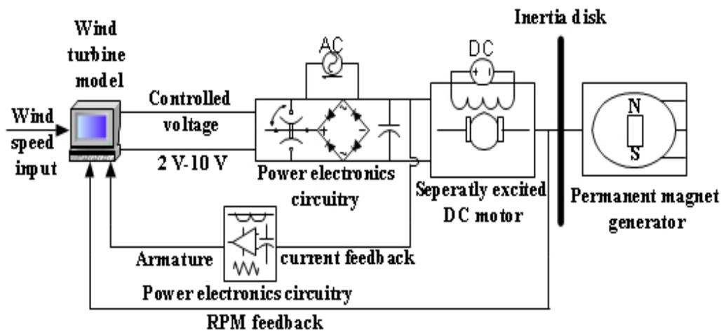
**Fig. 3:** Small wind turbine emulator structure
