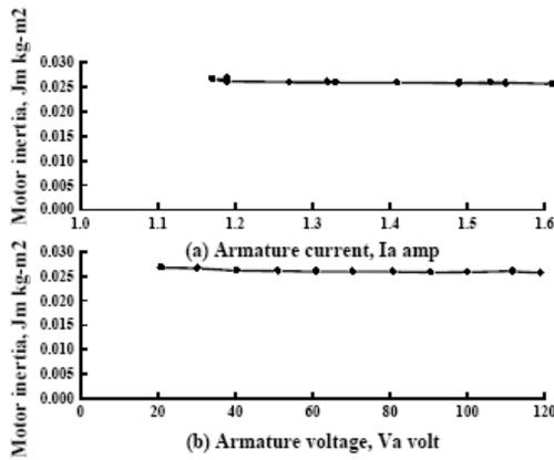
Fig. 7: Variation of motor inertia with armature (a) current and (b) voltage
