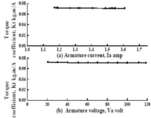
Fig. 9: Variation of torque coefficient with armature (a) current and (b) voltage
