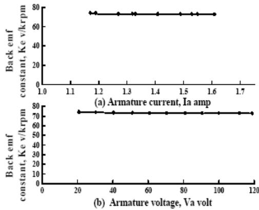
Fig. 8: Variation of back emf constant with armature (a) current and (b) voltage
