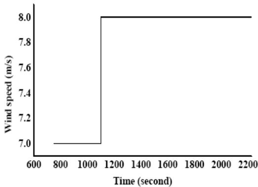
**Fig. 10:** Wind speed profile applied to the wind turbine emulator
