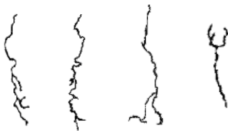
Figure 2. Surface tracking patterns of polymeric samples tested %40, %60, %80 and % 99 external moisture effects.
