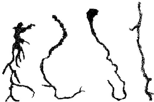
Figure 8. The samples under the fatigue effect (22 Hz and 8 hour longitudinal vibration)
