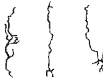
Figure 5. Surface tracking patterns of polyester samples tested under low (12Hz), medium (22Hz) and high (64Hz) frequencies.
