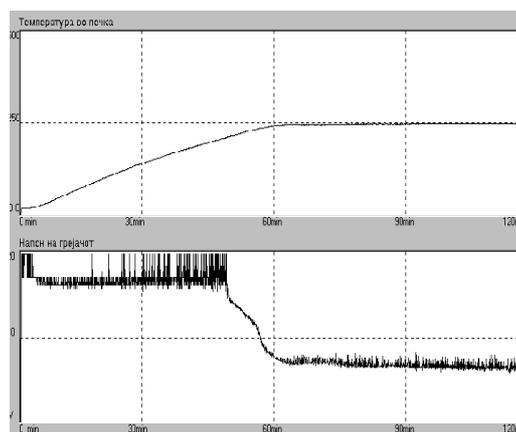
**Fig. 11** Initial results in terms of the actual responses of process temperature and heater voltage.
