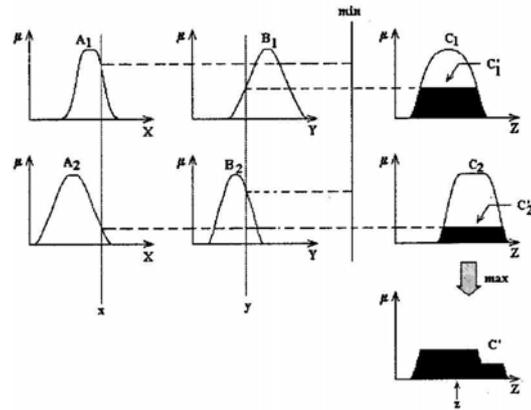
**Fig. 6** An illustration of Mamdani's fuzzy logic inference employed;  $X$  and  $Y$  are support fuzzy sets to error and change-in-error,  $Z$  is support fuzzy set to inferred control output.
