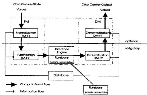
Fig. 4 Architecture of industrial fuzzy logic controller design employed for the prototype oven plant.
