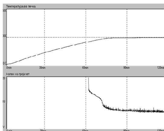
**Fig. 12** Actual heater voltage and temperature responses with the modified knowledge base
