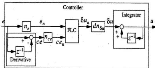
Fig. 3 Algorithmic system architecture of the generic fuzzy controller, represented by block 2 in Figure 1.
