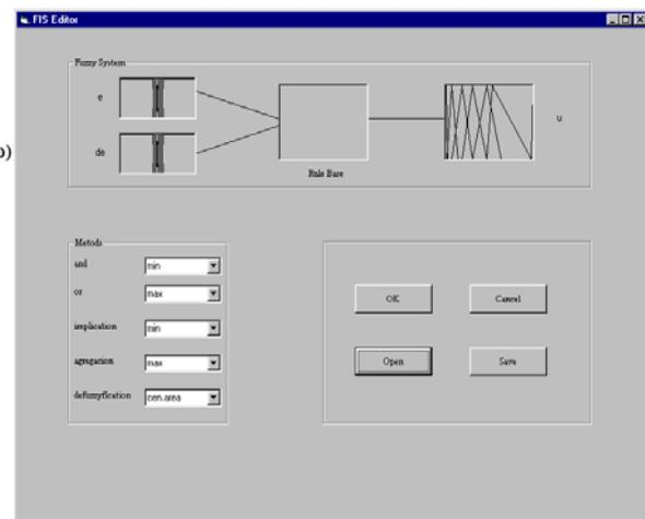
**Fig. 8** The window of the editor for designed fuzzy inference system.
