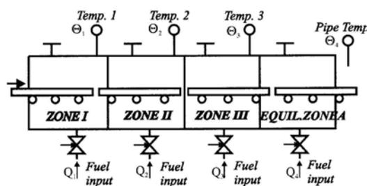
**Fig. 13** A schematic of a gas-fired, four-zone industrial furnace with disposition of transducers and actuators for temperature control.
