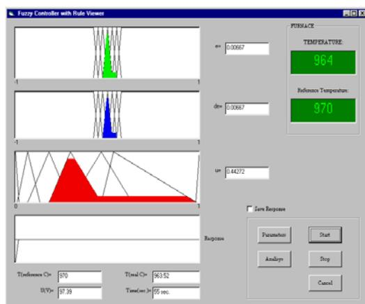
**Fig. 9** The window of fuzzy logic controller  $\delta u_n = FLC(e_n, ce_n) = f(e(t_n), \delta e(t_n))$  with fuzzy rule viewer module.
