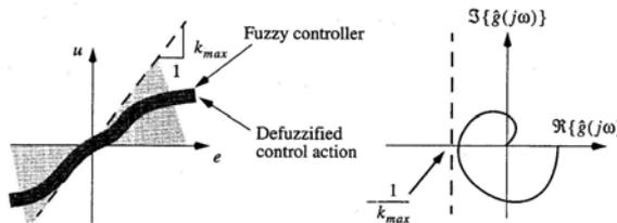
**Fig. 7** An illustration of the use of Popov's theorem in SISO fuzzy logic control systems.
