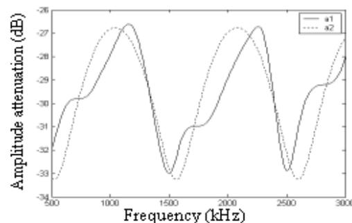
**Fig.1** Amplitude attenuation characteristics of measurement and model
