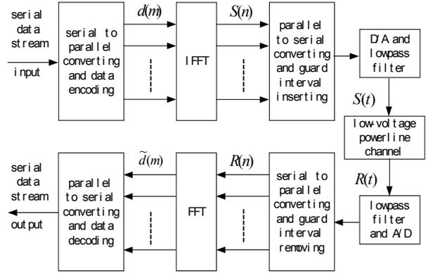
Fig.4 Block diagram of the OFDM based communication system
