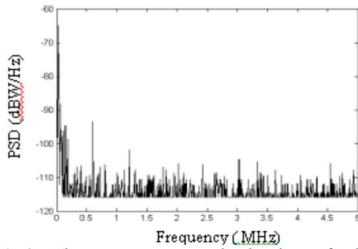
Fig.3 The power spectral density of the background noise
