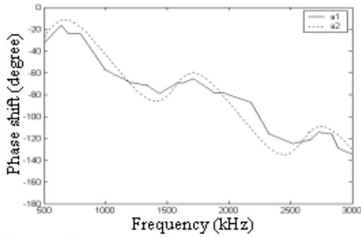
Fig.2 Phase shifting characteristics of measurement and model
