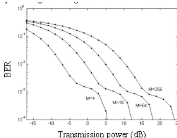
Fig.8 BER of the OFDM system
