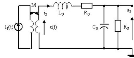
Fig. 4 Equivalent circuit for Rogowski coil
