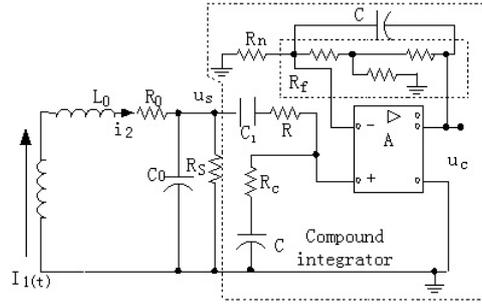
Fig. 5 Equivalent circuit for Rogowski coil with an outer integrator
