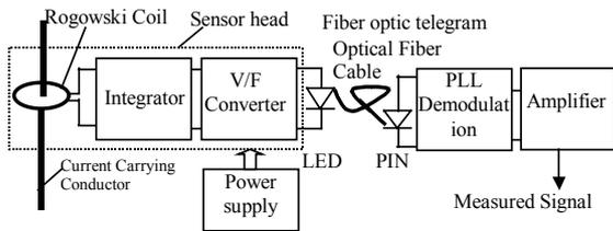
Fig. 2 Configuration of the opto-electronic current transducer
