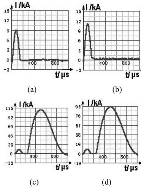
**Fig.7** Measurement results of currents of both preionization and primary discharge loop
