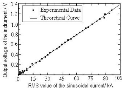
**Fig.5** Degree of linearity calibration of optic current sensor
