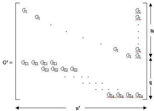
Fig. (3) EAPCC generator matrix [1].
