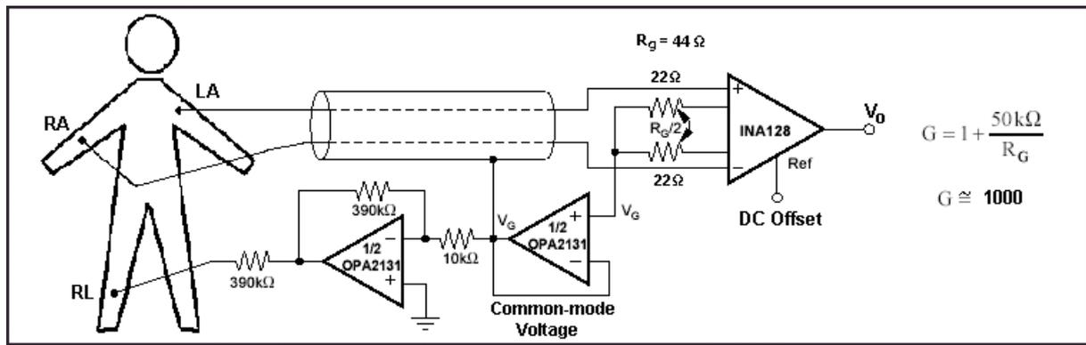
Figure 1. Instrumentation amplifier circuit
