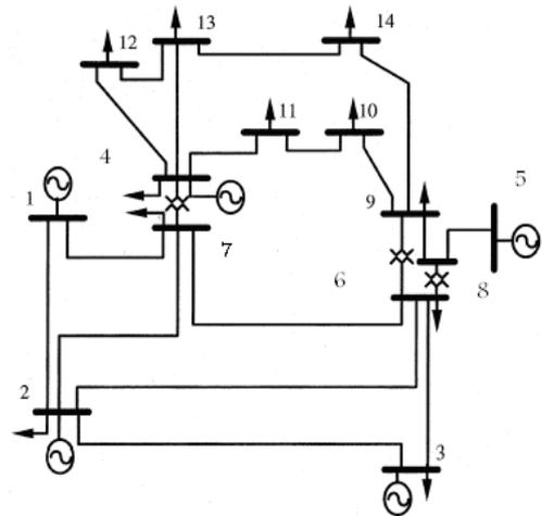
Figure 1. One line diagram of IEEE 14 bus test system.
