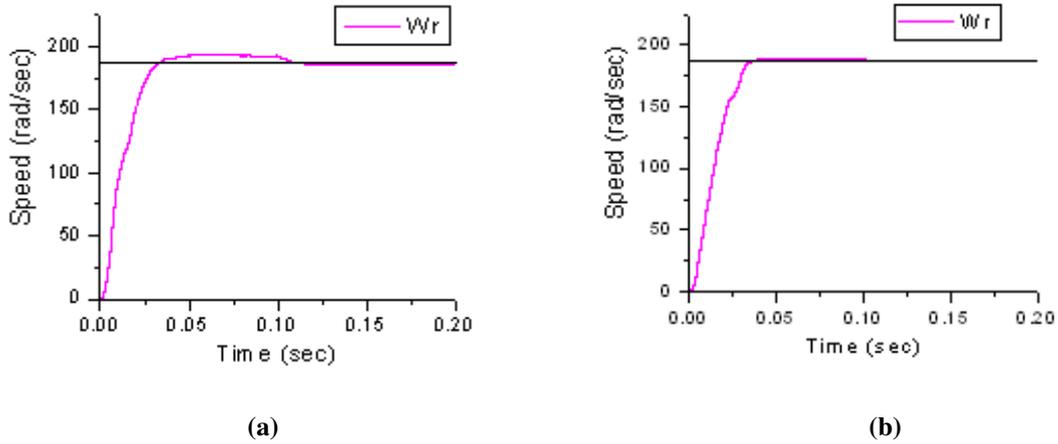
**Figure 11.** Speed responses for change in load torque. (a) PI, (b) FLC.
