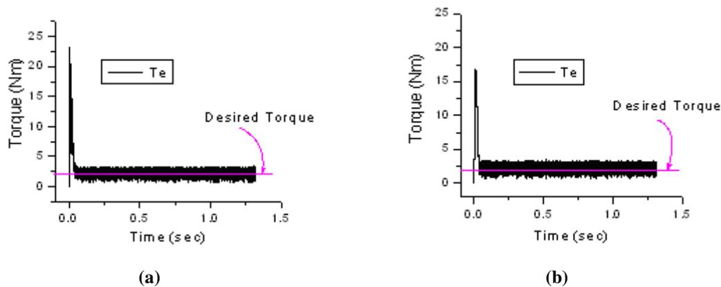
**Figure 8.** Developed torques of the drive system. (a) PI, (b) FLC.
