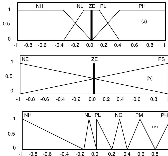
**Figure 5.** Membership functions for [7]: (a) Speed error ( $\Delta\omega_n$ ) (b) Change of speed error ( $\Delta e_n$ ) and (c) q-axis command current  $i_{qn}^*$ .
