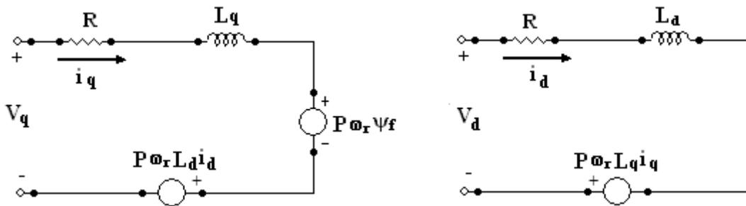
Figure 1. IPMSM d-q model
