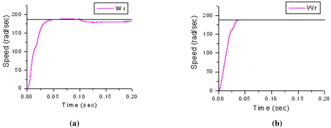
**Figure 12.** Speed responses with change of stator resistance (R to 2R). (a) PI, (b) FLC.
