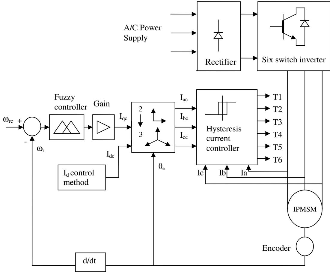
**Figure 3.** Control scheme of the IPMSM fed from a six-switch inverter.
