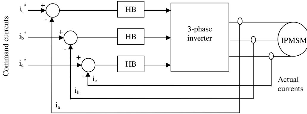
**Figure 6.** Hysteresis-Band (HB) current controller block diagram.
