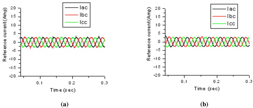
**Figure 9.** Three phase reference currents for (a) PI, (b) FLC.
