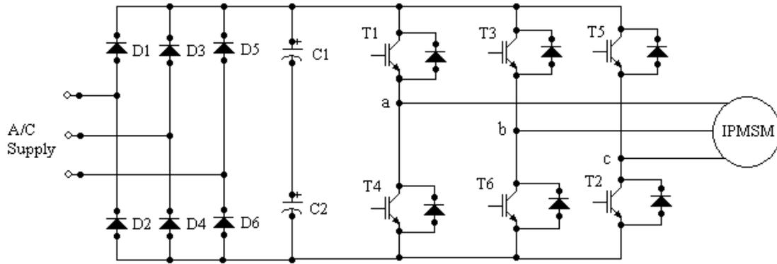
**Figure 2.** Power circuit of the drive system.
