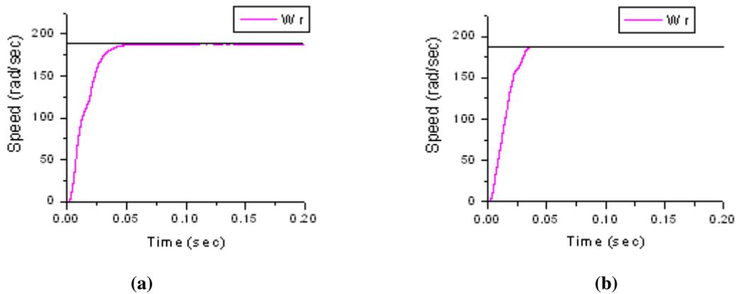
**Figure 7.** Simulated speed responses for the IPMSM drive at rated condition. (a) PI, (b) FLC.
