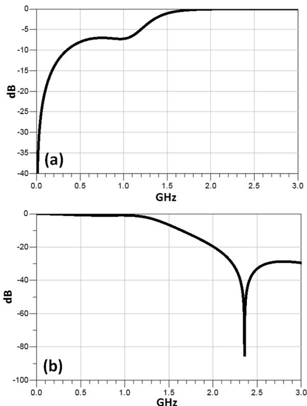
**Figure 4.** The return loss in (a) and the insertion loss in (b) for the designed stepped-impedance low-pass microstrip filter
