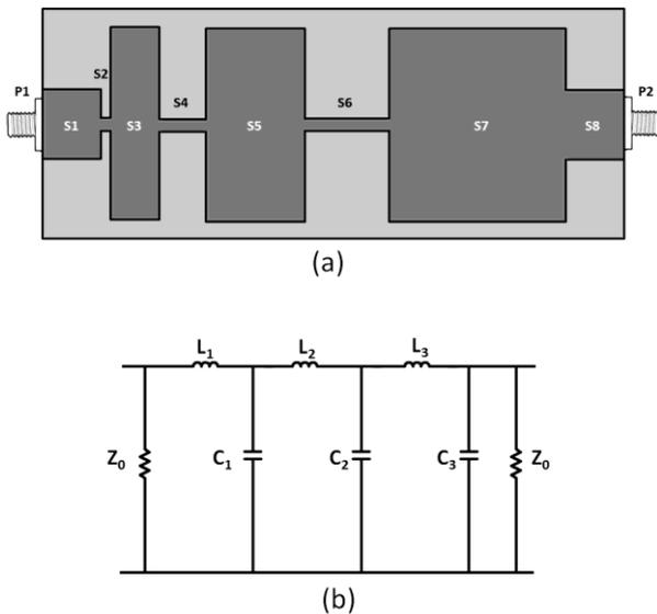
**Figure 2.** The designed stepped-impedance low-pass microstrip filter. The structure of the filter is shown in (a), while the L-C ladder type approximation of the filter is shown in (b)
