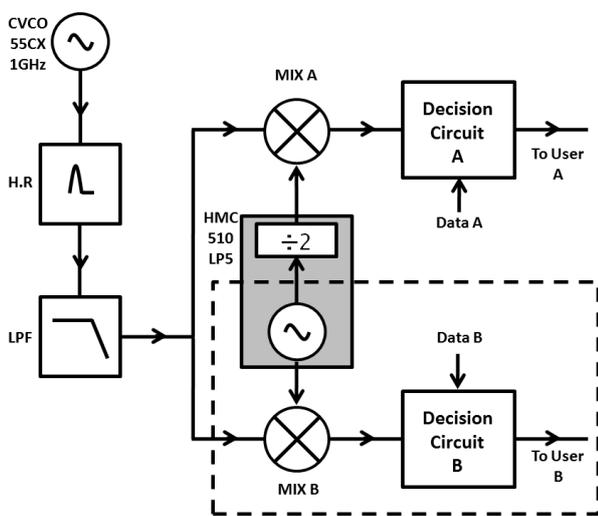
**Figure 3.** The first model of the designed pulse generator, including the extended part for FDMA which is surrounded by a dot-line
