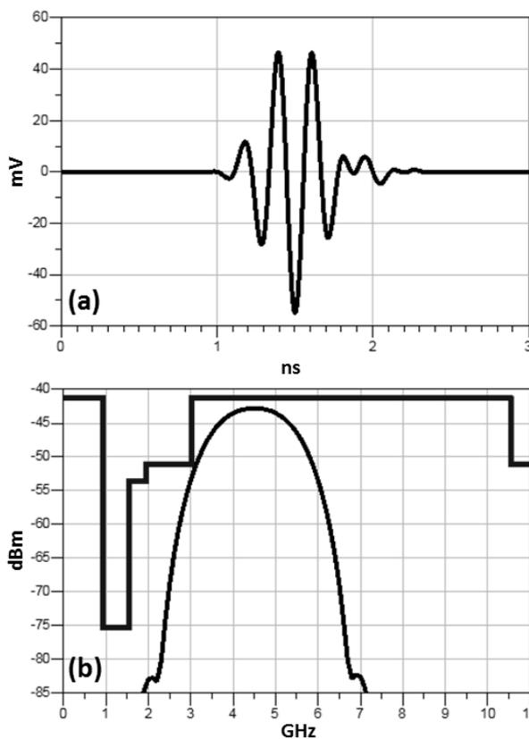
**Figure 5.** The up-converted pulse with 4.5 GHz in (a) time and (b) frequency domains
