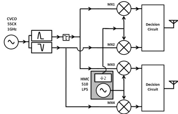
Figure 7. The second model of the designed pulse generator of 2 Gbps and 3 Gbps based on the decision circuit configuration and receiver setup
