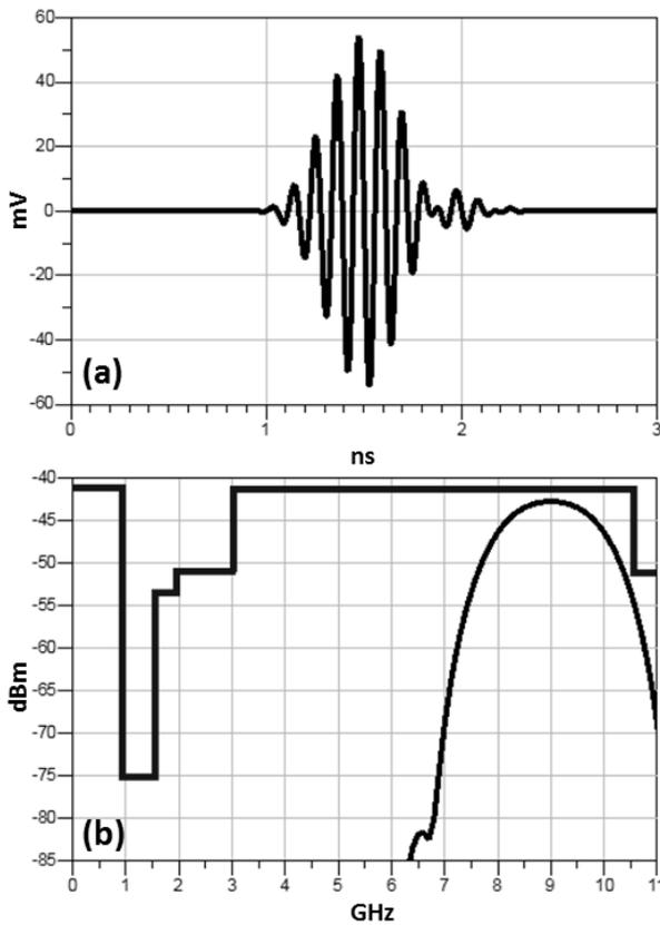
Figure 6. The up-converted pulse with 9 GHz in (a) time and (b) frequency domains
