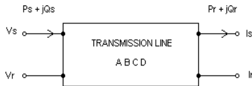
Figure 1: Two port four terminal model of a transmission line.
