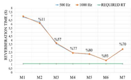
Figure A. Position of the panels used for model M6 (left), comparison of reverberation times of developed models (right)
