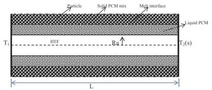
Figure 8. Schematic of the storage unit containing dispersed particles [42].
