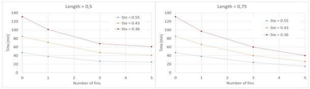
**Figure 3.**Total melting time as function of number of fins for different Ste number: 1=0.5(left), 1=0.75(right)[24].
