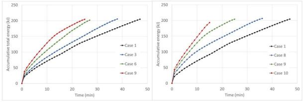
**Figure 4.**Accumulative energy as function of time at Ste=0.55: cases 1, 3, 6 and 9 (left), cases 1 and 8-10(right) [24].
