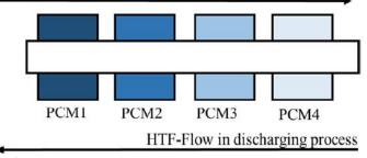
Figure 7. Schematic of multi-stage LHS system [28].
