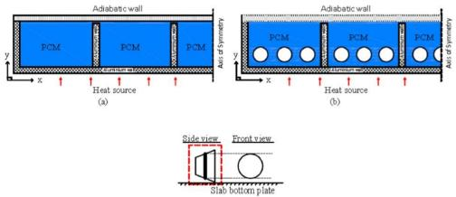
Figure 5. Two-dimensional simulation domain [25].
