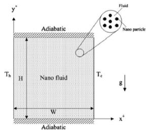
Figure 10. Schematic of a vertical enclosure system [45].
