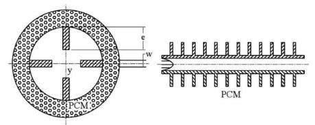
Figure 6. Schematic of internally and externally finned tubes deployed in [26] and [27].
