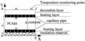
Figure 11. Configuration of the novel PCM floor [50].
