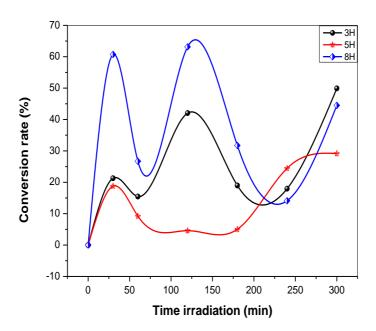
Fig. 4: Conversion rate of Methylene Blue by ZnO NRs with various deposition times
