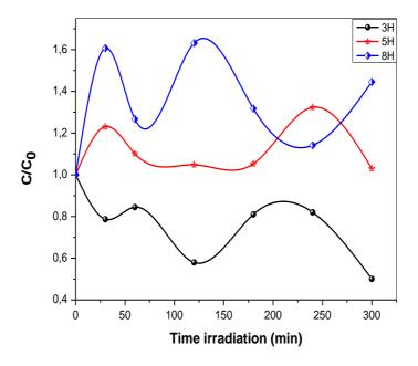
Fig.2: Photo degradation Kinetic of Methylene Blue by ZnO NRs with different deposition time
