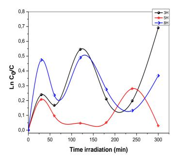
**Fig. 3:** Ln (C<sub>0</sub>/C) of Methylene Blue by ZnO Nanorods with various deposition times used a lamp with 254 nm
