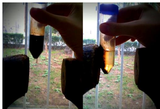
Figure 1. Magnetization of magnetic fructose imprinted polymer.
