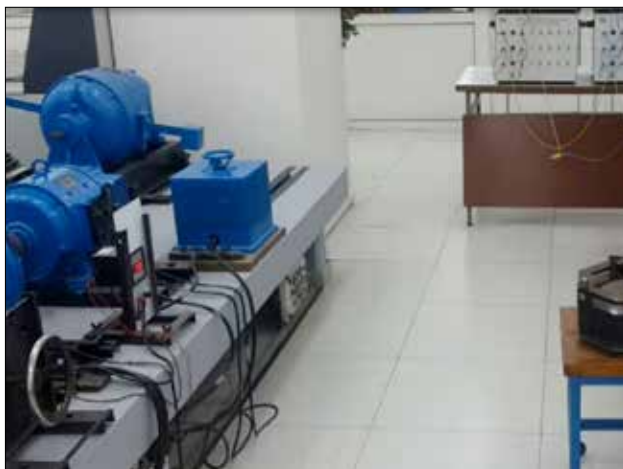
Figure 13. The set used for the tests for Supplying by Variable Frequency and Voltage
