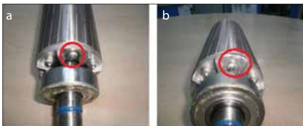
Figure 21. a, b. The rotor of test motor: serial production (a); without bearing balance spacer+ hammered(b); test setup (c)
