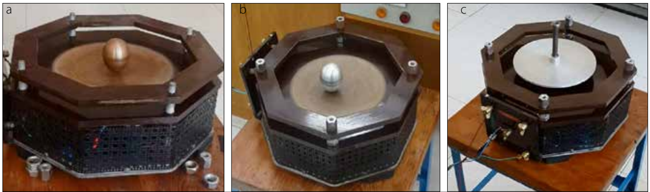
Figure 12. a-c. Rotational behaviour for different objects made of different materials in different geometrical shapes Copper egg (a); Aluminium egg (b); Aluminium disc (c)
