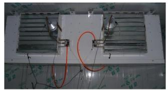
Figure 2. Schematic diagram of the air cooler with air pressure difference controllers.
