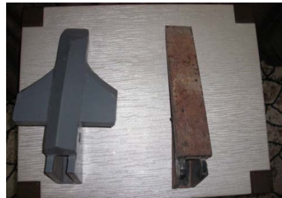
Fig. 6. Modified tine at left (with wings and angels) and Conventional tine at right of the image.
