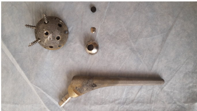
Figure 3: Asymmetrical wear of the metal head and the coin like free fragment originating from the head.
