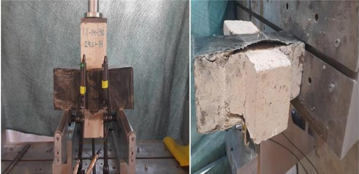
Figure 5. Specimen with De-bonding failure
