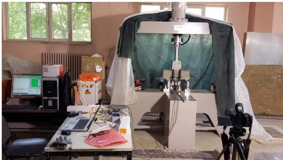
Figure 4. Corbel Specimen Setup
