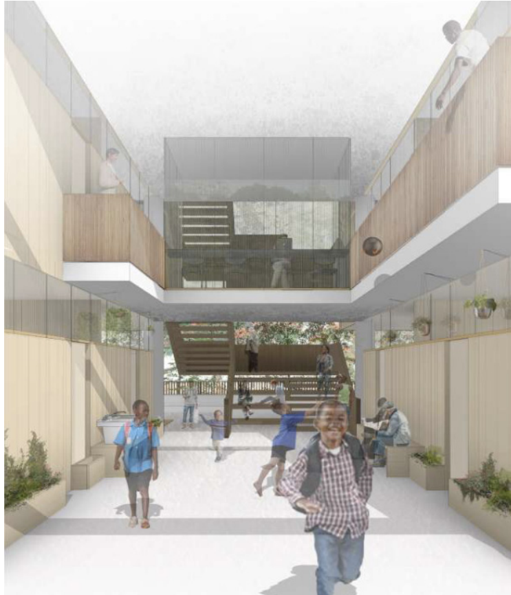
Figure 11. A perspective through a communal space demonstrates how an existing concrete frame office building can be transformed by inserting sustainably sourced timber elements (Madolo, 2017).
