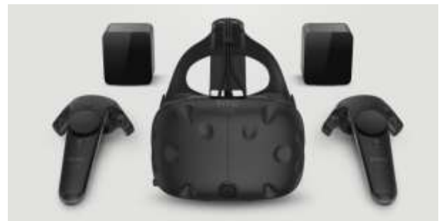
Figure 7. HTC Vive main components [19]
