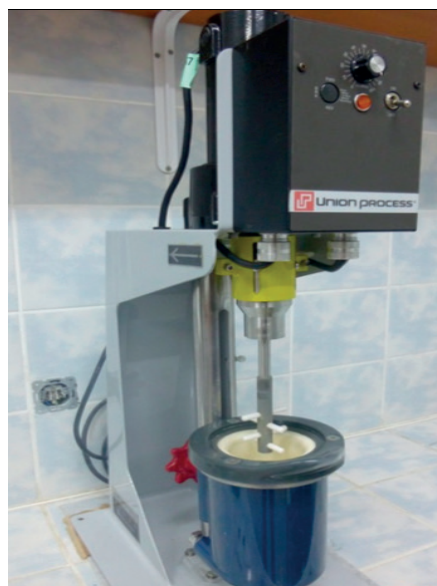
Figure 3. The stirred mill used in the ultra-fine grinding (UFG)
