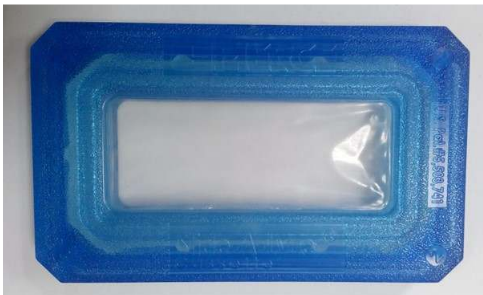
Figure 2. Dialysis cassette; 2000 MWCO and 3 – 12 mL capacity.
