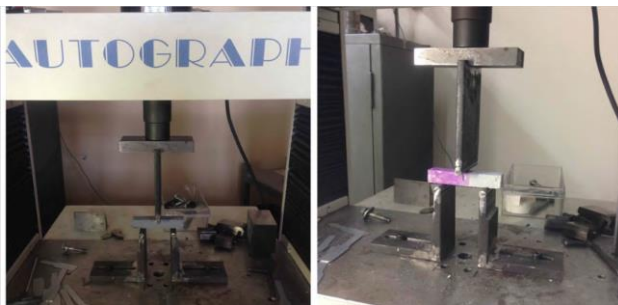
Figure 8. Destructive evaluation test, 3 Point bending test, to evaluate mechanical strength enhancement, [25]
