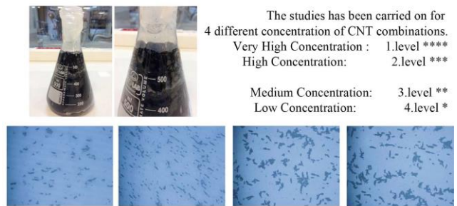
Figure 9. Effect of colloidal stability on CNT dispersions before application to samples of building material, searching the effect of Carbon nanotubes on mechanical strength of construction materials, [25]
