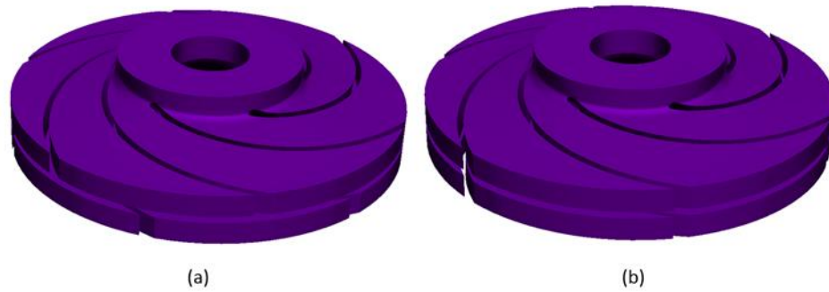
Figure 4. Three-dimensional geometry of staggered (a) and non-staggered (b) impeller
