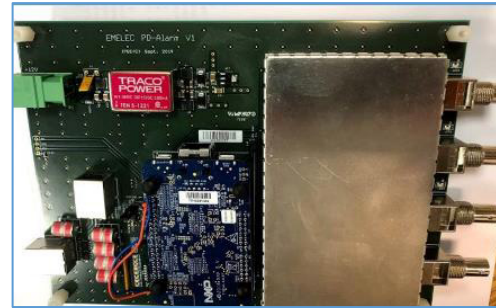
Fig. 3: PD measuring board including 3 input channels, a input sync. channel
