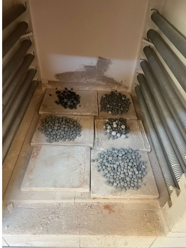
Figure 3. Sintering process of ALAs
