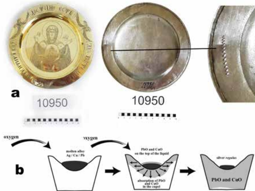
Figure 4: Coupling Scraping Lines on a Mercury Plating (Amalgam) Coated Silver Plate (a) and Schematic Illustration of the Coupling Process (b) Photograph: Şirin KAYA and Irmak Güneş YÜCEİL; Diagram (Torres, Thomas, and Aude Mongiatti, 2008: p. 60)
