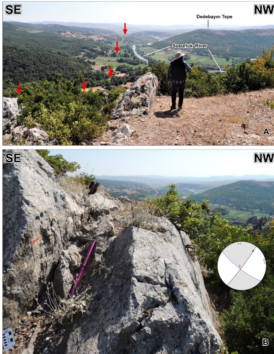
Figure A.34. A) Position of SHF-2a from Karaköy to Aziziye. Note the systematic shear fractures on the Paleozoic-Triassic recrystallized limestone which is parallel to the SHF-2a. B) Close-up view of the shear fracture with kinematic data. The circle represents the equal area lower hemisphere spherical projection of the fault plane and slicken-lines. Gray and white areas (contractional and extensional areas, respectively) are the fault plane solution obtained by kinematic analysis of the fault data. The 1, 2, and 3 indicate the orientation of kinematic (strain) axes (after Seyitoğlu and Esat, 2022a).
