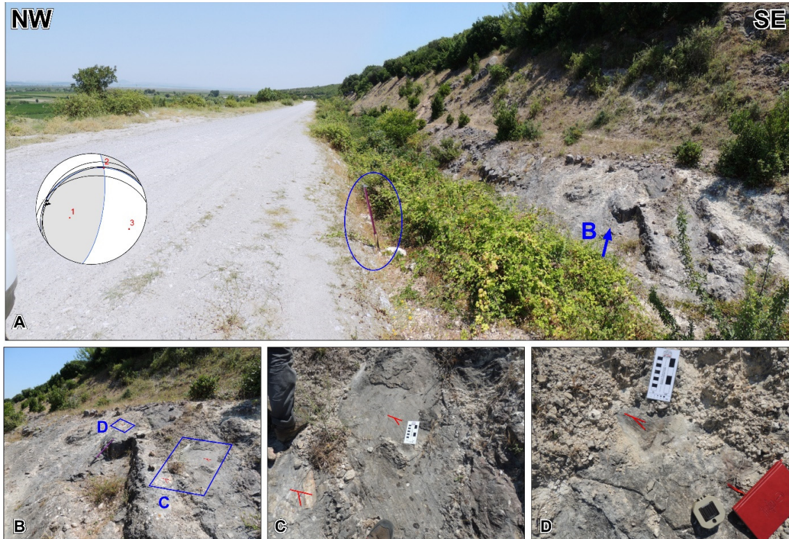
Figure A.27. A) The bending area of DDF-1b in the south of Ulubat Lake. B, C and D) details of kinematic data (after Seyitoğlu and Esat, 2022a). The circle represents the equal area lower hemisphere spherical projection of the fault plane and slicken-lines. Gray and white areas (contractional and extensional areas, respectively) are the fault plane solution obtained by kinematic analysis of the fault data. The 1, 2, and 3 indicate the orientation of kinematic (strain) axes.
