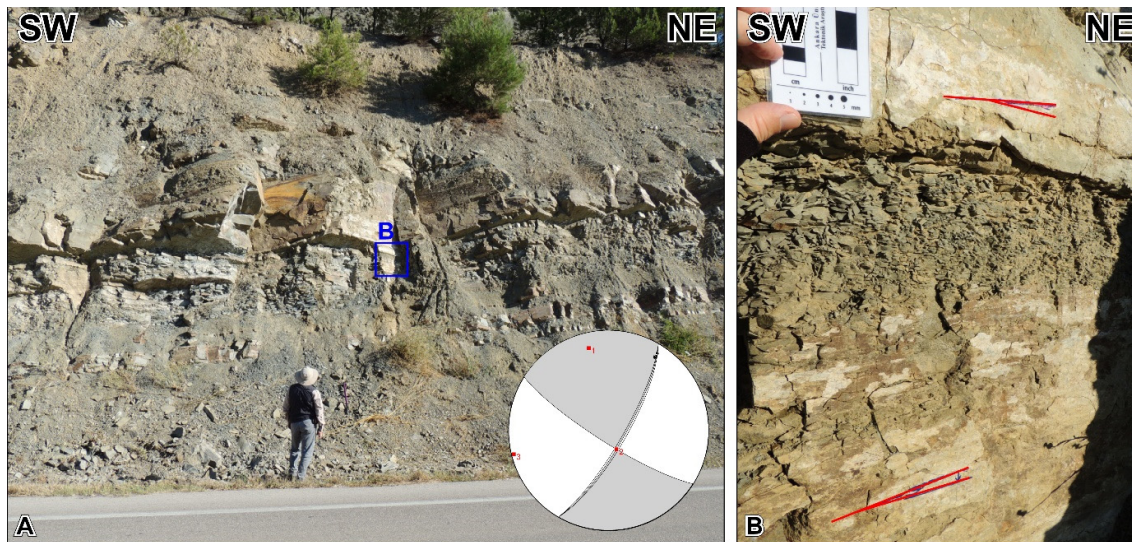
Figure A.8. A) Systematic shear fractures in the Cretaceous marl and shale alternation provides kinematic data in the linear valley where MDF-6f is located. B) Close-up view of the shear fractures. The circle represents the equal area lower hemisphere spherical projection of the fault plane and slickenlines. Gray and white areas (contractional and extensional areas, respectively) are the fault plane solution obtained by kinematic analysis of the fault data. The 1, 2, and 3 indicate the orientation of kinematic (strain) axes.
