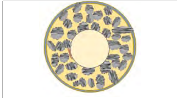
Figure 6- Invasion of the unconsolidated formation by the high gel mud.
