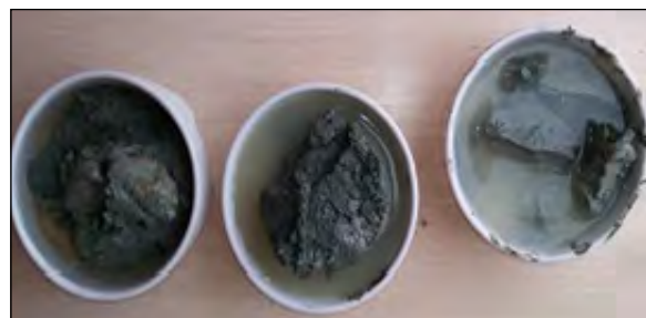
Figure 7- Keeping the core samples in mud and water and observation of the properties such as dispersion and swelling.
