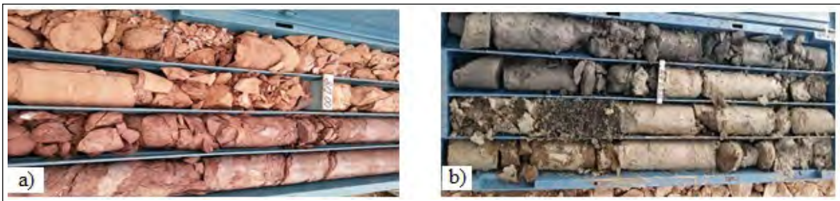
Figure 1- a) Brittle mudstones encountered in the Terzili and Yörüklü areas and b) unconsolidated sandstones, claystones and siltstones in the Suluova field.
