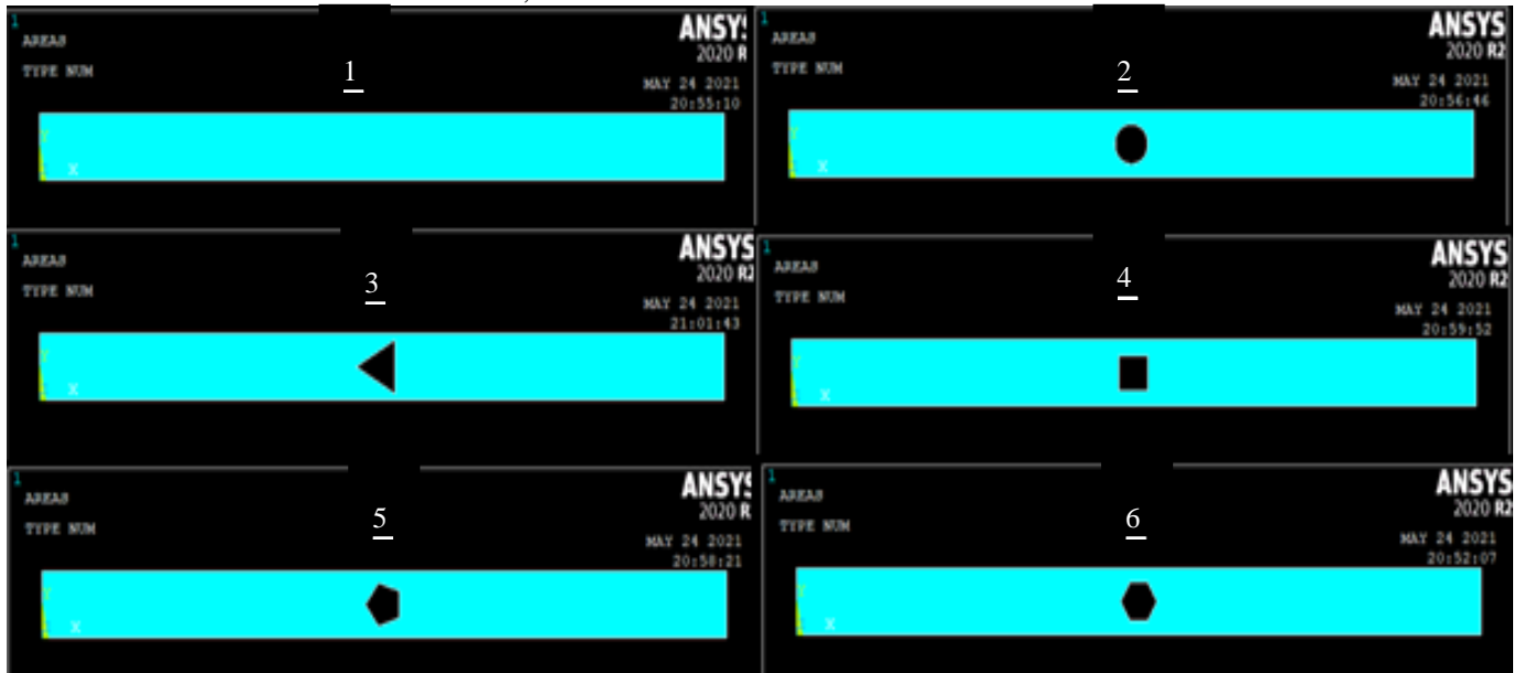
Figure 1 A schematic model of a sandwich structure. 1) no cutout, 2) circular cutout, 3) triangular cutout, 4) rectangular cutout, 5) pentagonal cutout, 6) hexagonal cutout.
