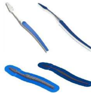
Figure 1 The solid model and parting line of the molded two-component toothbrush
