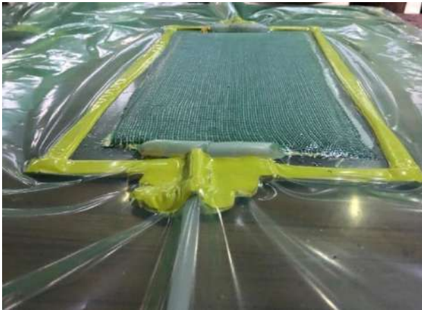
Figure 5 Vacuum assisted resin transfer molding process
