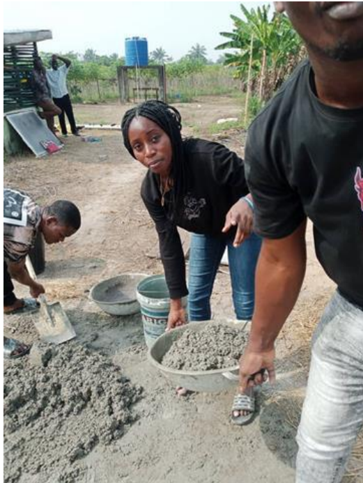
Figure 4. Taking of fresh concrete for laboratory analysis.
