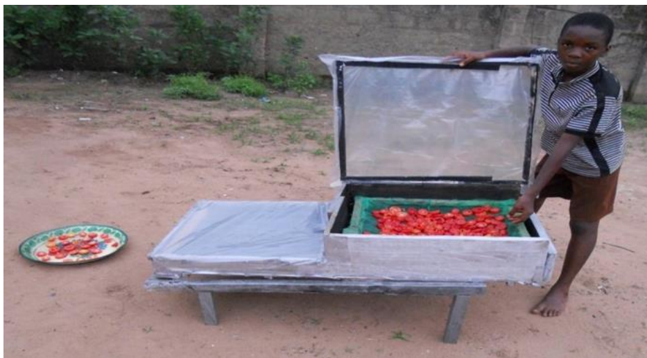
Figure 16. Solar dryer constructed with wood solar thermal collector ( Eke, 2014 ).
