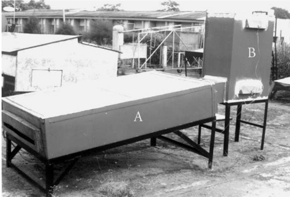
Figure 7. The air heating system (A-collector assembly with energy storage and air-heating subsystems; B-heated space) (Enibe, 2001).
