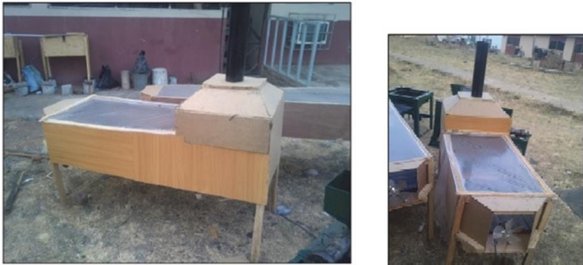
Figure 24. The indirect-active desiccant solar crop dryer (Itodo et al. , 2019).
