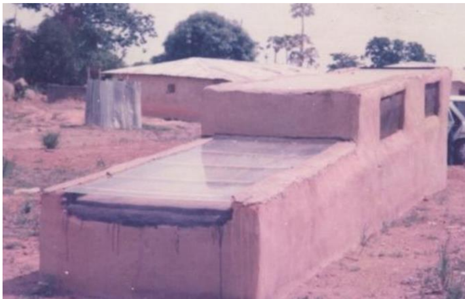
Figure 17. Solar dryer constructed with cement thermal solar collector ( Eke, 2014 ).
