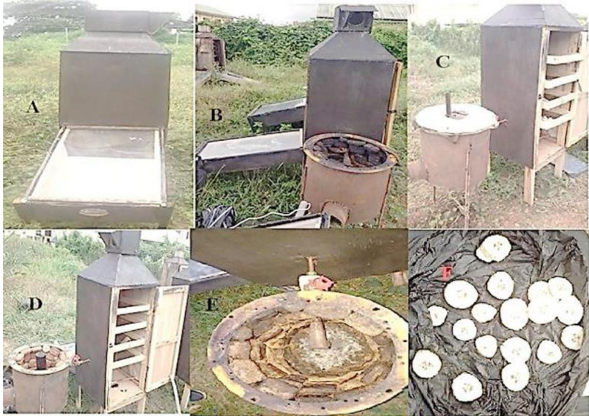
A-solar dryer without biomass heater; B-side view of the array of the two solar dryers with the biomass heater furnace open; C-solar dryer showing the biomass heater furnace covered and the door open; D-the biomass heater with the cylindrical pipe in place to create the flue gas duct during feedstock loading; E-biomass furnace revealing the connection of the exit pipe into the combustion chamber; F-sun drying of the plantain slices
