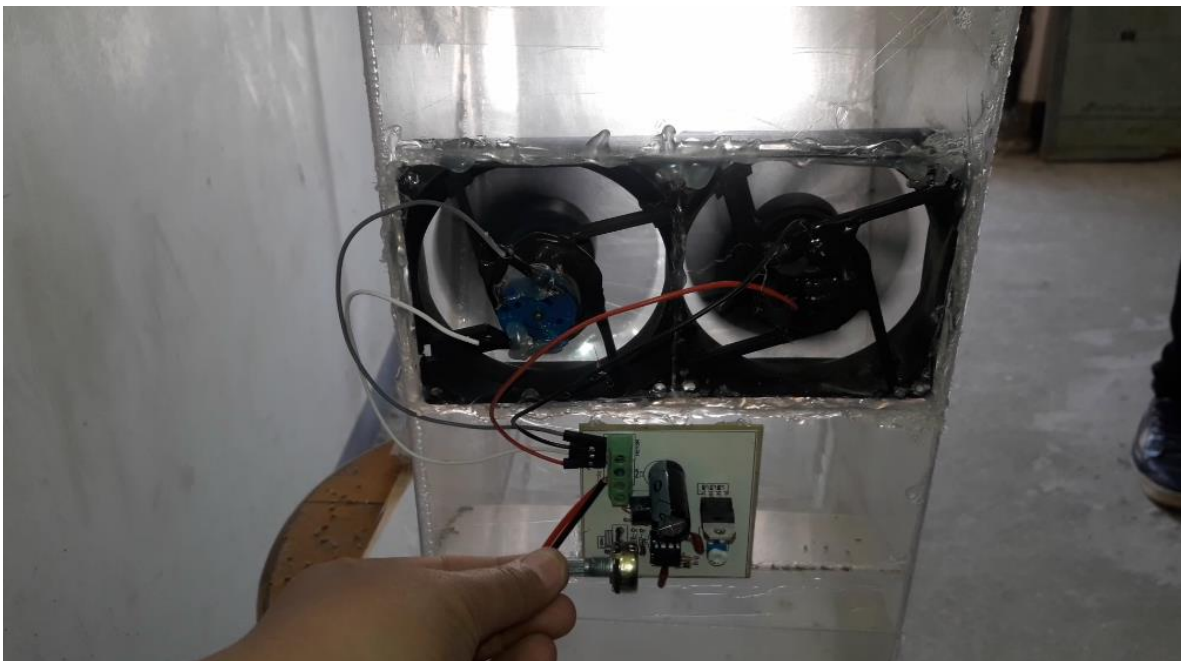
Figure 2: Blast fans and switch.
