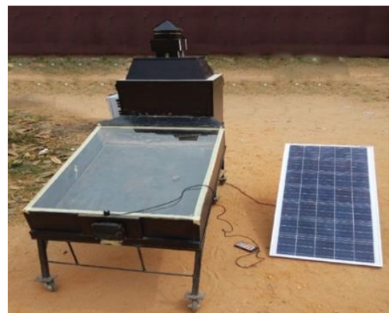
1-Temperature/Humidity sensors; 2-Exhaust fan; 3-Door frame; 4-Drying racks; 5-Weighing balance; 6-Iron bar (support); 7-Battery/Inverter assembly; 8-Solar collector; 9-Inlet fan; 10-Plain glass; 11-Screw bolt; 12-Drying chamber hood; 13-Chimney; 14-Cable; 15-Heating element; 16-Roller.
