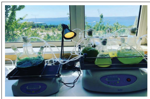
Figure 1. Microalgae adhesion test of the composite coating.
