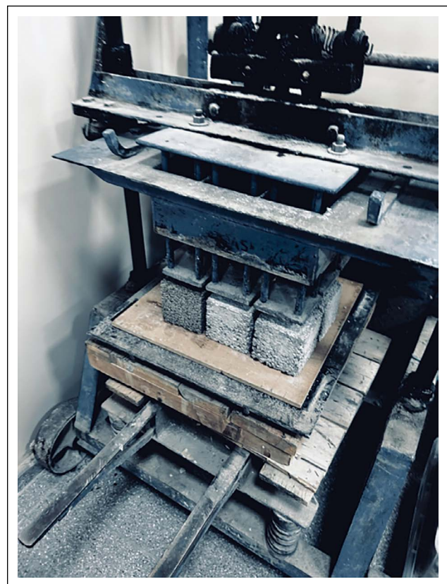
Figure 2. Cubic specimen production process.
