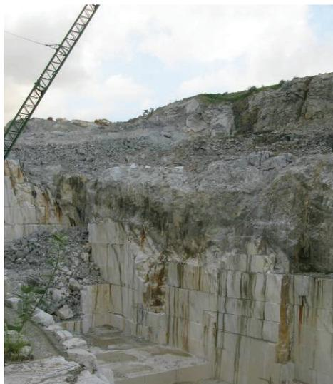
**Figure 3** - Waste material to be removed to carry out the exploitation of the white marble underneath, Ambaji quarry, Gujarat (India).
