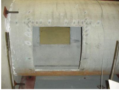
Figure 3. Diametrically opposite large openings of the chimney section [3]
