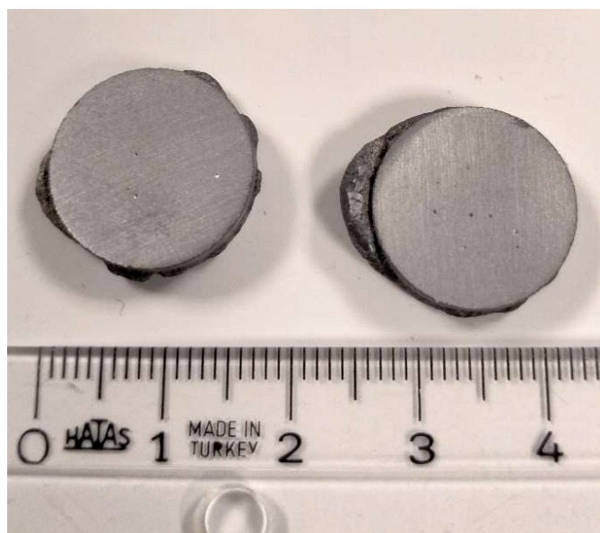
Figure 3. Furnace Sintered at 650^\circ\text{C} (Left), Sintered at 700^\circ\text{C} (Right) Relatively Molten Pure Aluminum
