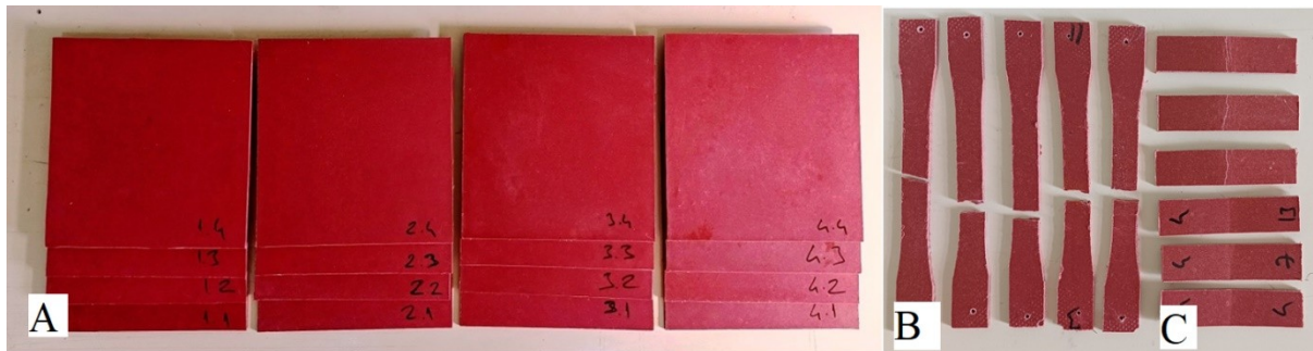
Figure 2. Composite boards (A), Tensile test samples (B), Flexural test samples (C)
