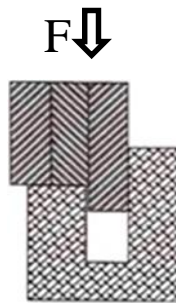
Figure 5. Shear strength test parallel to fibers and glue line
