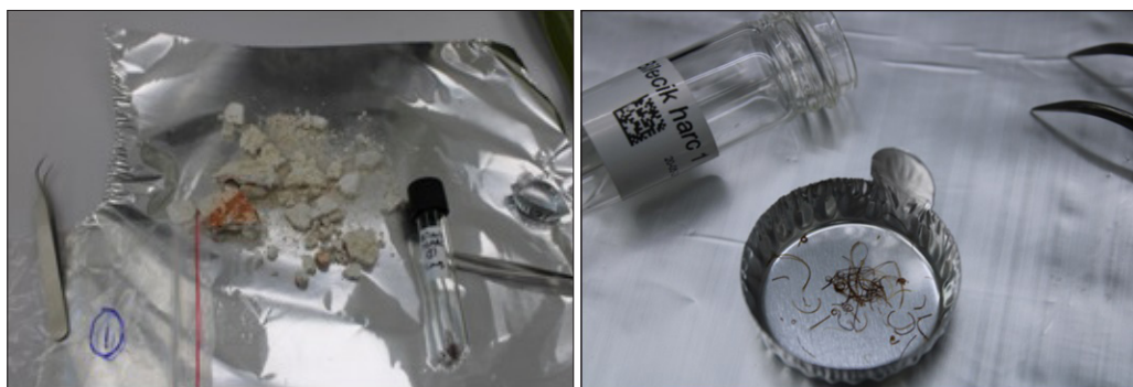
Figure 10: Mortar Sample Sampled (a), Sample of Completed Physical and Chemical Cleaning Process (b).
