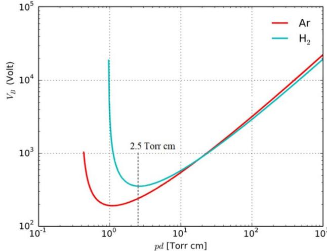
**Figure 7.** The  $P \cdot d$  product corresponding to 2.5 Torr.cm, marked on the Paschen curves of Ar and H<sub>2</sub> gasses [3].
