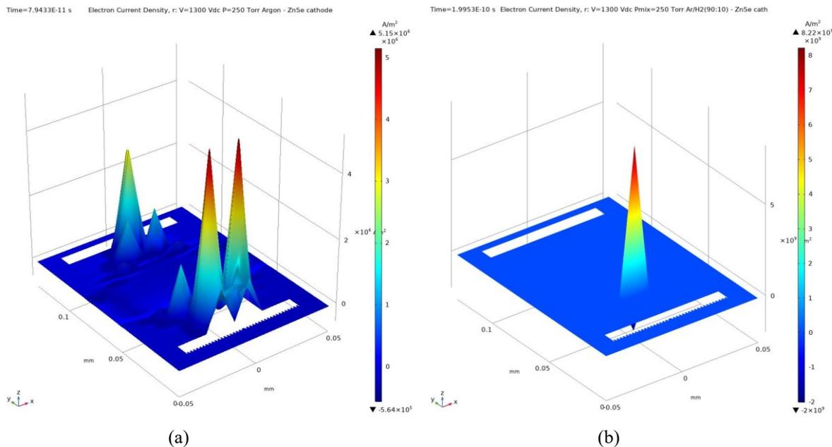
**Figure 5.** Spatial distributions of electron current density (ECD) data obtained across 100  $\mu\text{m}$  long discharge gap in 3D images, respectively for; (a) final phase of unary Ar -system, (b) final phase of binary Ar/H<sub>2</sub> (90:10) -system.
