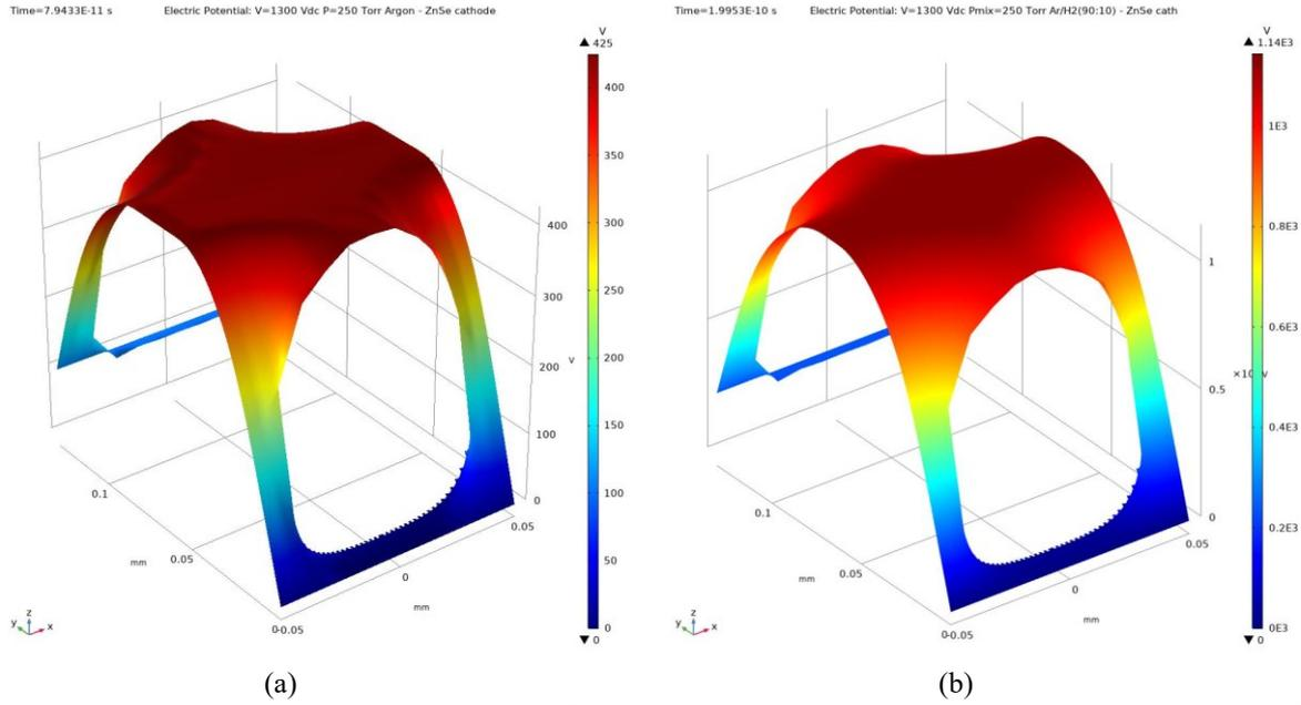
**Figure 6.** Spatial distributions of electric potential (EP) data obtained across 100  $\mu\text{m}$  long discharge gap in 3D images, respectively for; (a) final phase of unary Ar -system, (b) final phase of binary Ar/H<sub>2</sub> (90:10) -system.
