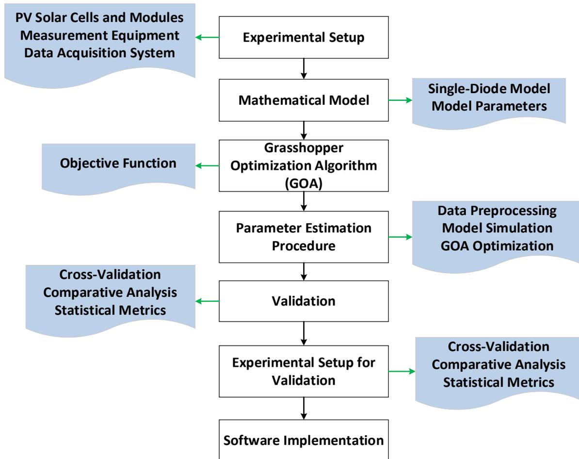
**Figure 1.** Grasshopper-based parameter extraction for PV module
