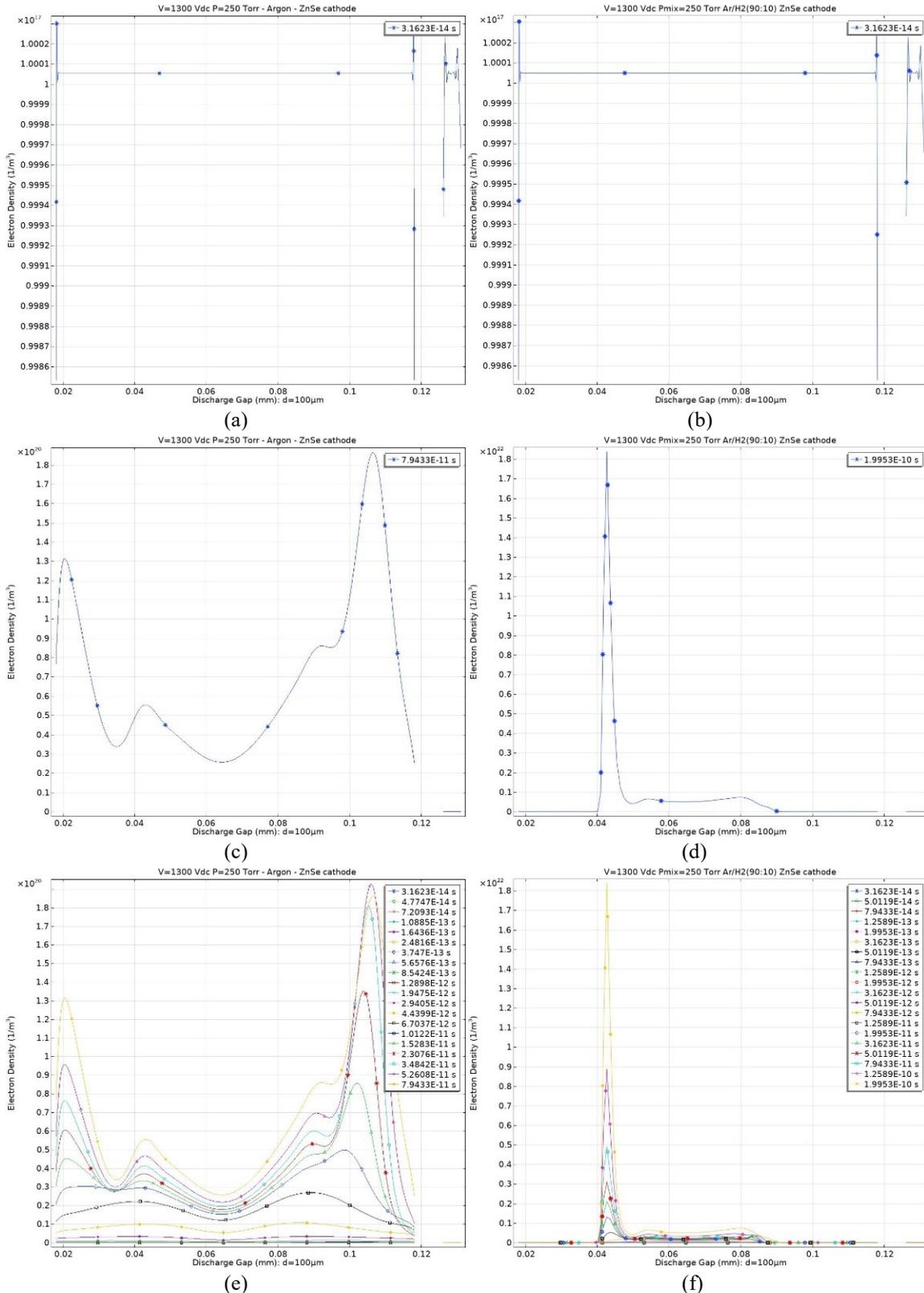
**Figure 3.** Spatiotemporal distributions of electron density (ED) data across 100  $\mu\text{m}$  long discharge gap, respectively for; (a) initial phase of unary Ar -system, (b) initial phase of binary Ar/H<sub>2</sub>(90:10) -system, (c) final phase of unary Ar -system, (d) final phase of binary Ar/H<sub>2</sub> (90:10) -system, (e) full period of unary Ar -system, (f) full period of binary Ar/H<sub>2</sub> (90:10) -system.
