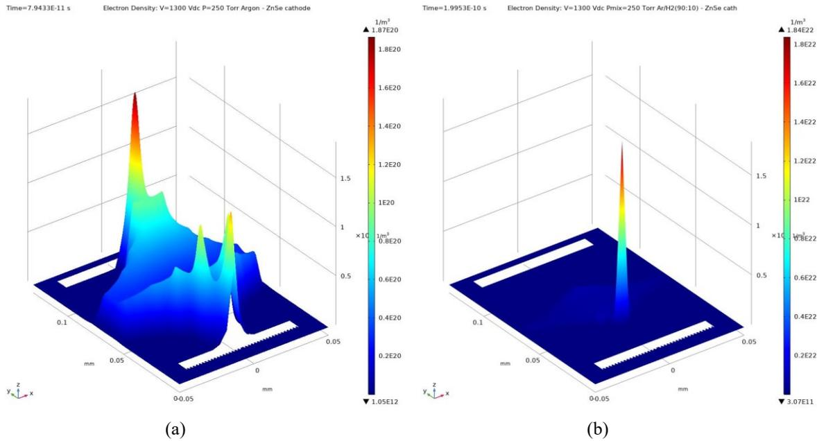
**Figure 4.** Spatial distributions of electron density (ED) data obtained across 100  $\mu\text{m}$  long discharge gap in 3D images, respectively for; (a) final phase of unary Ar -system, (b) final phase of binary Ar/H<sub>2</sub> (90:10) -system.
