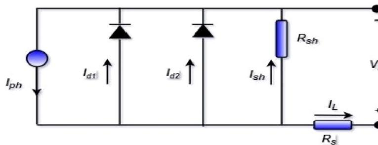
**Figure 3.** Equivalent circuit of the DDM model
