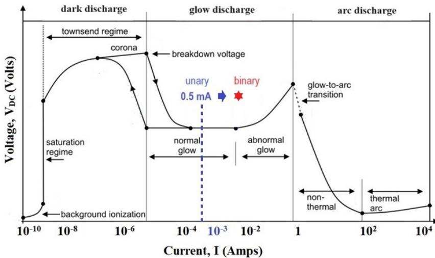
**Figure 8.** Peak discharge currents of unary Ar and binary Ar/H<sub>2</sub>-discharge systems, lying in the normal glow discharge regime of the V-I curve [13].
