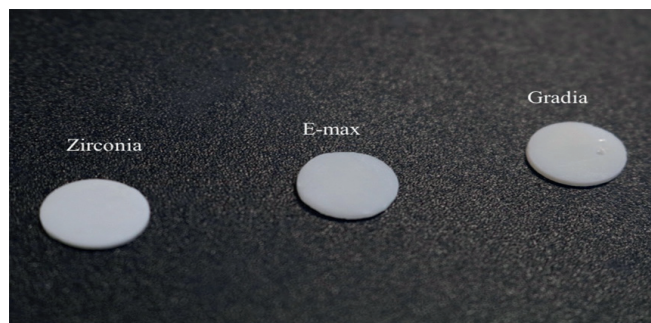
Figure 1: The final shape of the disc materials (Zirconia, E-max and Gradia)
