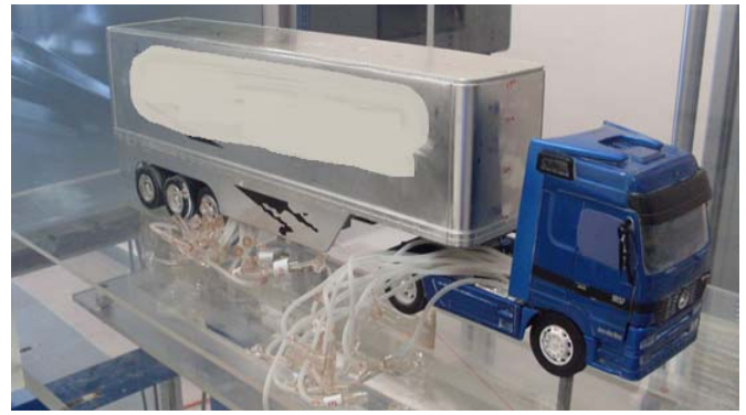
Fig.2a. The locations of the pressure probes on model vehicle
