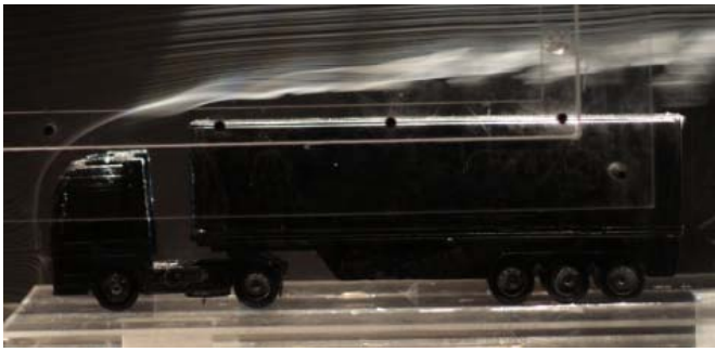
Fig.6. Flow separations around base model truck-trailer (Bayindirli et al. 2016)
